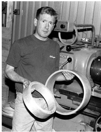
Patrick Cooperman holds wood hoops that will become a drum and banjo rim. Cooperman's lumber is locally harvested and sawn at the company mill.
